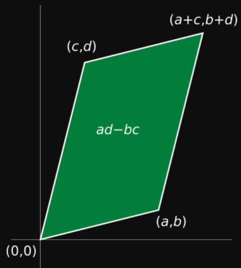
$$\det \begin{pmatrix} a & c \\ b & d \end{pmatrix} = \text{signed area of parallelogram}$$
