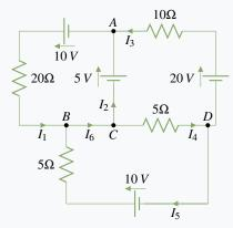
First apply the junction rule at junctions *A*, *B*, *C*, and *D* to obtain
