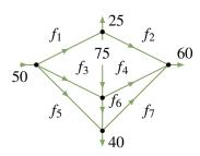
**Exercise 1.4.2** A proposed network of irrigation canals is described in the accompanying diagram. At peak demand, the flows at interchanges *A*, *B*, *C*, and *D* are as shown.
