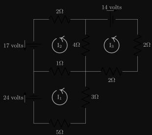
The equation for the bottom circuit, with current  $I_1$  is given by
